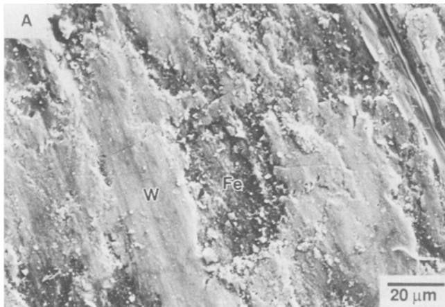
Fig. 8 Surface morphologies of the counterpart steel ring for ring-on-square adhesive wear test. (a) Material A. (b) Material D
