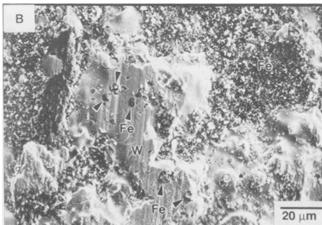
Fig. 9 Surface morphologies of ring-on-square adhesive wear test. (a) Material A. (b) Material D
