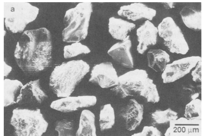
Fig. 1 Feedstock powders of WC-12Co plasma spray material. (a) As-received powder morphology. (b) Cross-sectional view of as-received powders
