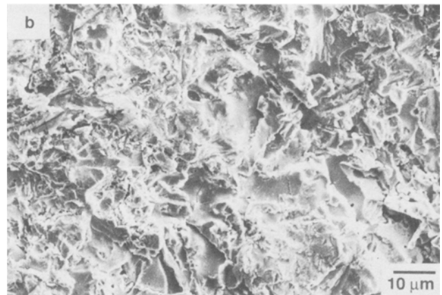
Fig. 13 Erosion scar of plasma-sprayed WC-12Co coating. (a) 90° impact of specimen B. (b) 60° impact of specimen B. The arrow in the mid-view of (a) indicates either fracture at a splat boundary or fracture that is associated with porosity.
